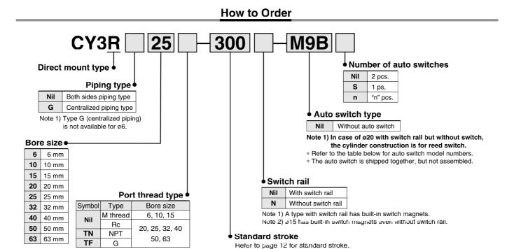
Applicable Auto Switches/The applicable auto switch is determined by the bore size. Heter to pages 21 to 23 for further information on auto switches.
