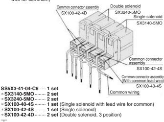
The asterisk denotes the symbol for assembly. Prefix it to the part nos. of the solenoid valve, etc.
