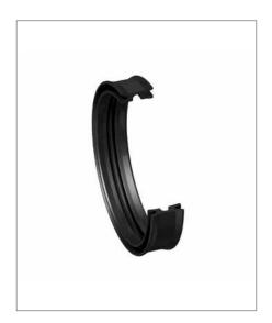
The Z5 pneumatic piston seal is a double U-ring with an integral guiding surface for double-acting pistons. The seal has two sealing lips for particularly high sealing performance.
