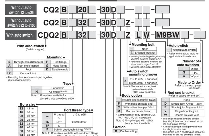
Note 3) "TF" is not available for air-hydro type. Refer to the next page and \* For cylinders without auto switch, M threads are page 3 for standard strokes compatible only for ø32-5 mm stroke. and intermediate strokes.
