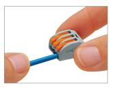
3. Lower the lever to close the clamp to complete the connection.4. To remove, lift the lever and pull out the conductor.
