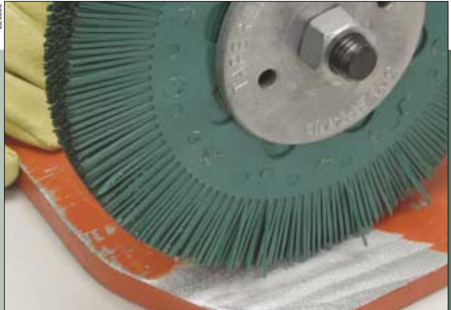
8" Radial Bristle Brush, grade 50, removing paint from straight shaft tool.
