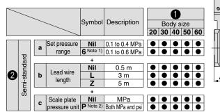
Note 1) Set pressure range of 6P(L, Z) is 0.2 to 0.6 MPa (30 to 90 psi). Note 2) This product is for overseas use only according to the new Measurement Law. (The SI unit type is provided for use in Japan.)
