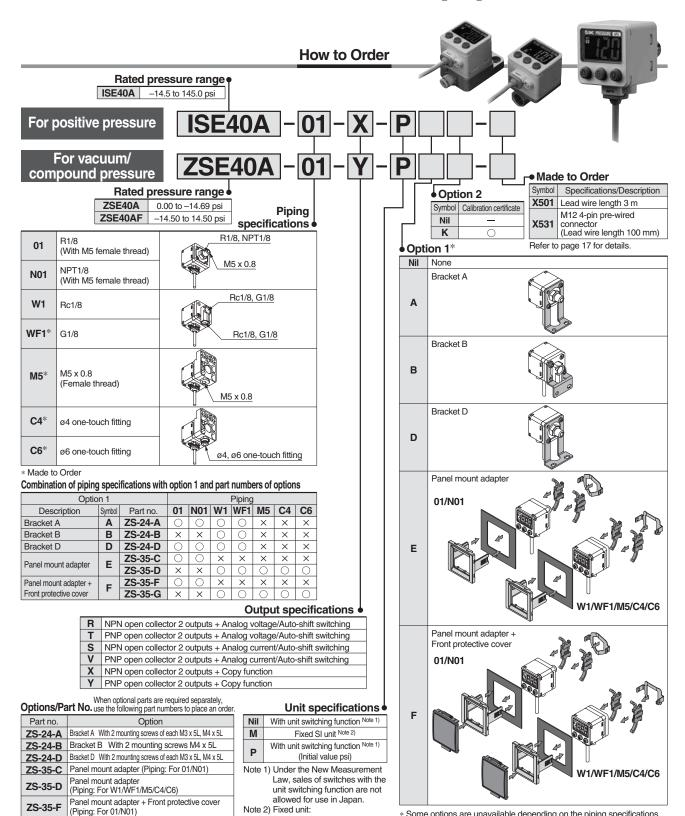
Some options are unavailable depending on the piping specifications. Refer to "Combination of piping specifications with option 1 and part numbers of options". . For positive pressure: MPa
