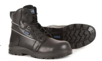
**Characteristics** Dual density PU sole resistant to oils and hydrocarbons. Profile wrapping for stability in the march deep crampons, self-cleaning and multi directional. Synthetic material safety cap protecting a shock of 200 Joules. Non-metallic anti-perforation midsole complies with standard 12568: 2010, full protection of the foot. Weight: 715 g (weight from one foot in size 42)
