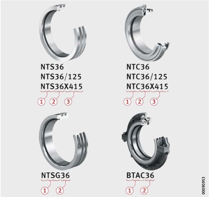
Figure 19 Designation structure of standard seals, examples
