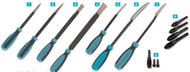
Hand scrapers are designed for the removal of high spots on machined surfaces to give a smoother surface on slideways, bearings, cast iron surface plates and precision marking out plates. All scrapers have a soft feel handle and are made from high grade tool steel suitably hardened, to maintain a very keen cutting edge
