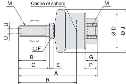
\* Use the precision spanner for clock 4 mm in the case of mounting male thread of JS10.
