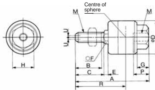
Use the precision spanner for clock 4 mm in the case of mounting male thread of JA6 and JA10.
