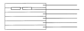
Protective Film (polyester 50 Print Adhesive Carrier Film (polyester 12u) Adhesive Double coated siliconized pa
