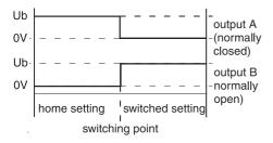
This switch is used to monitor **one** switching point. When the switching point is reached, exit A (port 4) closes, which corresponds to the normally closed type. Meanwhile, exit B (port 2) changes to the flow state, which corresponds to the normally open type.
